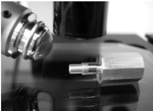
FIGURE 4 – CoCr cylinder in place for microscopic analysis
